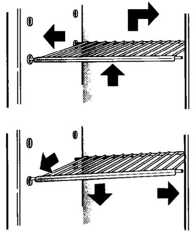
**NOTE:** The shelf should lower slightly and lock into place. If the shelf does not appear sturdy, make sure both ends of the shelf are inserted into the shelf support cups.
