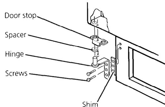
**NOTE:** When replacing the doors, set the door gap at 17 mm ( $\frac{1}{16}$ ”).
